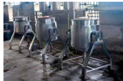
Picture 2: Concentrated solar thermal-based steam cooking system implemented by A.T.E. Enterprises Private Limited at NLC Dahanu
