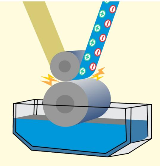
Electrostatically charged films and paper can create a potentially hazardous situation in solvent based laden coating or printing stations, especially in winter. Static discharges occur through an electric spark, which in solvent-vapour laden areas can be hazardous.
