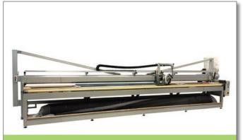
T650 (6.5 meter active shearing width)
