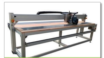
T300 (3 meter active shearing width)
