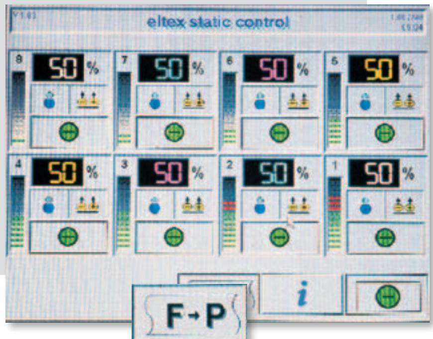
The electrostatic printing assist works equally well for paper as well as film. Simply use the appropriate key on the remote control panel to switch over manually to film operation.
