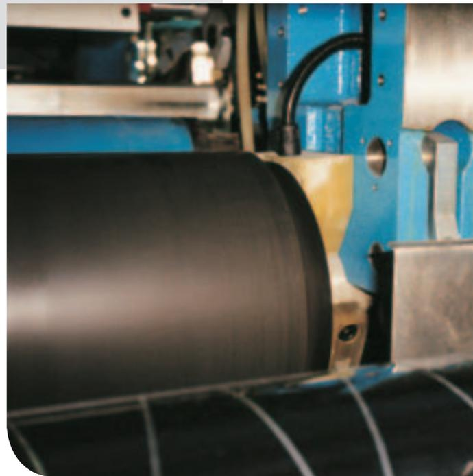
**The GNH61-System** is designed for installation in any gravure printing press. The work involved includes installing the charging and discharging bars, installing and connecting the generators, installing the remote control and wiring the system. Typically, a packaging gravure printing press with six or eight printing units can be fully ESA-equipped and ready for operation within one weekend.
