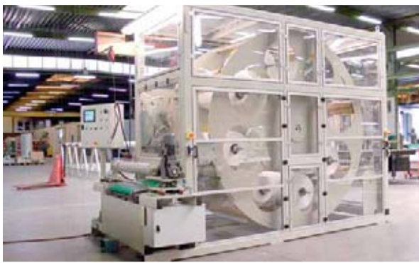
Multilayer fabric tube assembly machine Unwinding station for multiple fabrics with integrated cut-to-size unit and ultrasonic welding for the production of fabric tubes.
