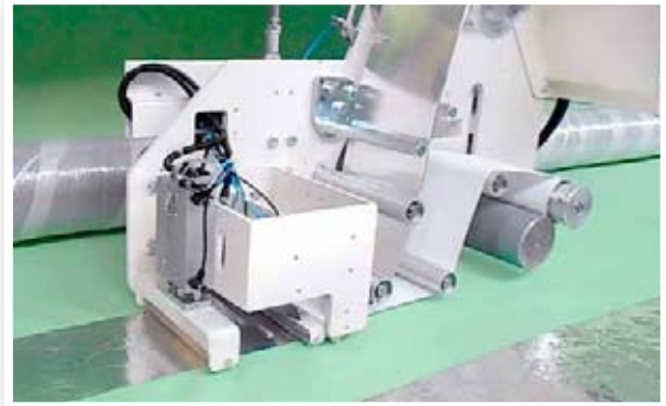
Applicator for aluminium tape onto needlepunch non-woven
