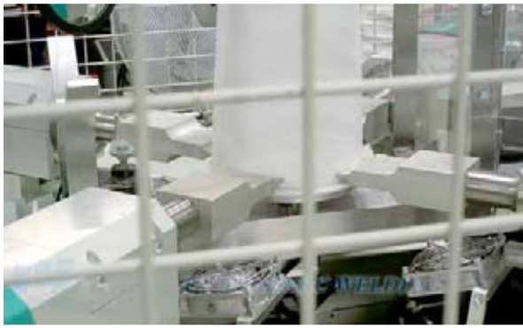
Ultrasonic welding of filter bags onto plastic rings
