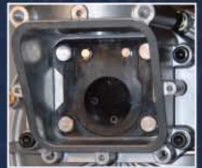
Four bolts release valve cover for service
